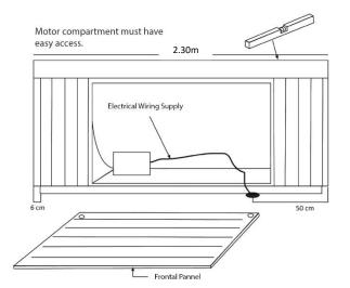
**IMPORTANT:** Important: The equipment must be connected to an exclusive and permanent power line capable to support installed power. Lighting and electrical receptacles must be located at least 1.5 meters from the equipment.
